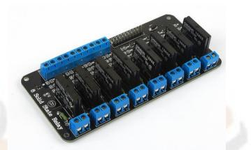
This 5V 2A 8-Channel SSR G3MB-202P Solid State Relay Module is based on the G3MB SSR relay which can control up to 2A at 240VAC. This is an 8 Channel SSR relay module, each relay channel has 3 separate terminals, NO (Normal Open), COM (Common), NC (Normal Closed).
